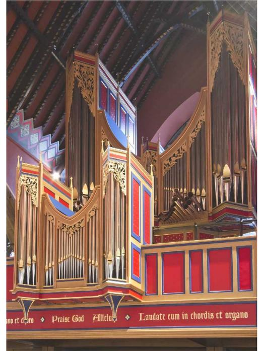
The organ was built as new by Kenneth Tickell at his Northamptonshire workshops using state-of-the-art CFC machining facilities and the slides demonstrated the care and expertise involved in great detail. Assembly and case design were fascinating and the positioning of the copper-based *en chamade* trumpet pipes in a case of tin-rich display pipes was of especial interest to some of us. The quality of the wood for pipes was absolutely top-class.
